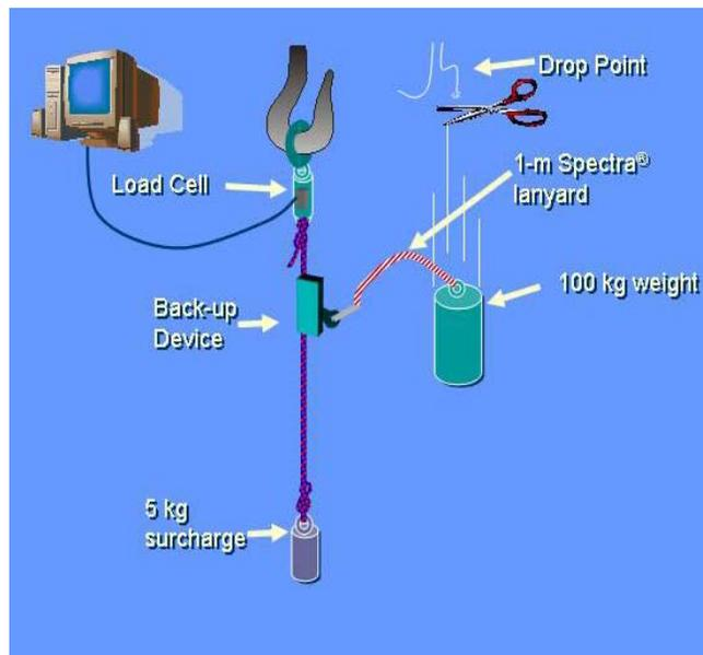
The load cell, connected to a data logger, was placed at the anchor (crane lifting hook). Each rope was attached to the load cell with a pre-tensioned figure 8 knot. All the knots were adjusted by the same person applying approximately 30 kg of force to set each knot. Each device was placed on a marked spot 60 cm below the anchor point.
