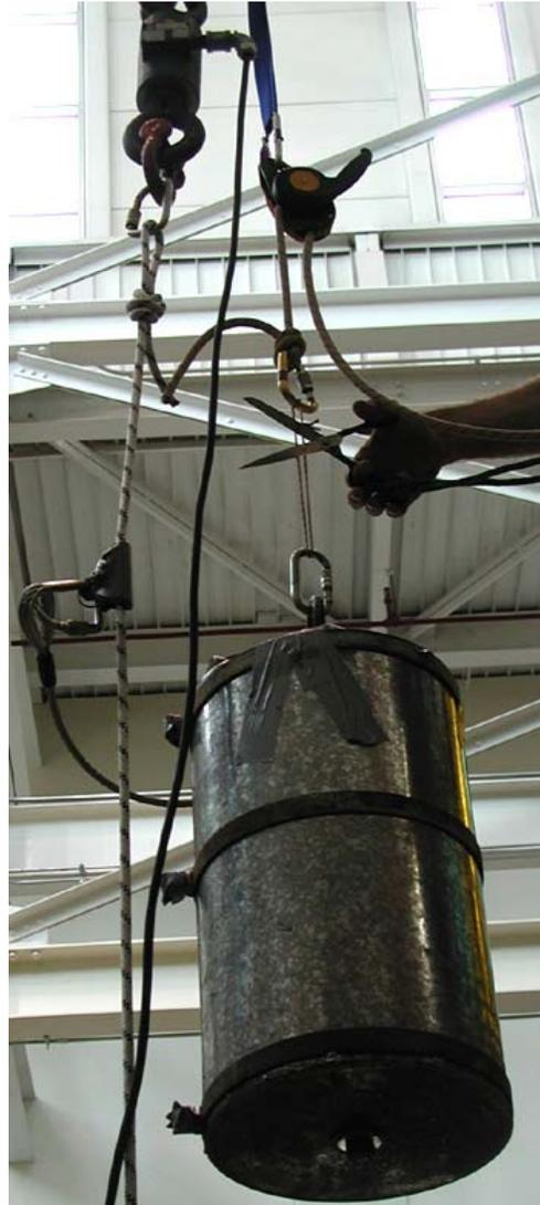
Figure 3: Factor 1, 100 kg test rig
